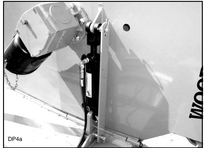
Figure 2. Transport Lock-Up Bar - Right Wing
